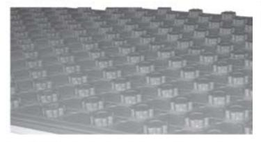
NOTE: The panels are divided into 3" squares. Each square either contains a knob or a flat and they alternate every other square. When placing the first panel of a new row you must check to verify that from row to row, this alternating sequence of knob-flat-knob-flat is not interrupted. Otherwise it could cause difficulties when laying the PERT tube later on.
