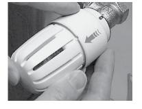
Then, without tools, slide the locking sleeve 3 towards the hand wheel until the hand wheel scale is covered and the sleeve clicks into position.
