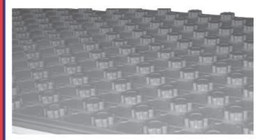
NOTE: The panels are divided into 3" squares. Each square either contains a knob or a flat and they alternate every other square. When placing the first panel of a new row you must check to verify that from row to row, this alternating sequence of knob-flat-knob-flat is not interrupted. Otherwise it could cause difficulties when laying the PERT tube later on.
